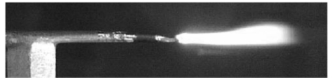
Fig. 15 Appearance of a deeply subcritical MW discharge, initiated by a thin sharpened vibrator, in supersonic airflow. The vibrator is supported in the middle part by a streamlined holder.
