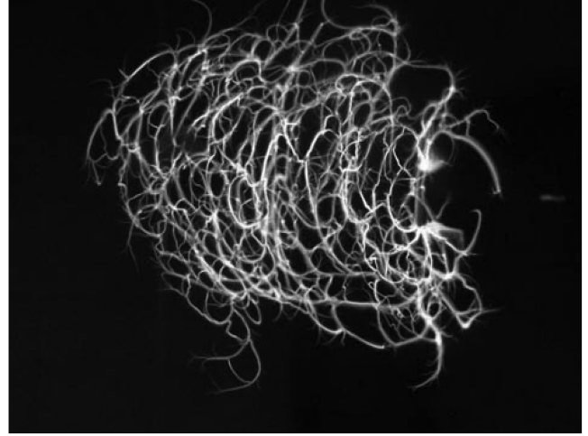
Fig. 4 Photograph by open lens of the volumetric subcritical MW discharge; MW radiation is directed from left to right; pulse duration of MW radiation is 40 \mu s , air pressure is 760 torr, wave length is 8.9 cm, and length of the initiator is 2 cm.
